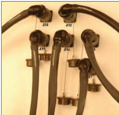
▲ Fig. 1 SQ-8 multipin connectors can be fitted in compact areas.
